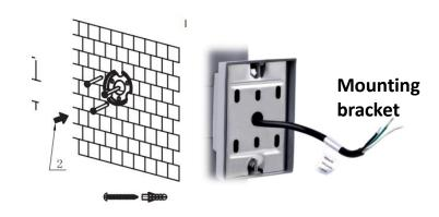
2)Fix the mounting bracket on the mounting face with 4PCS self-tapping screws
