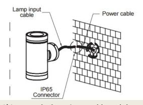
3)Connect the lamp input cable and the power cable
