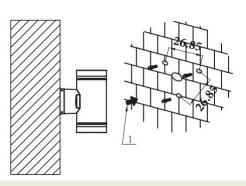
1)Drill 4 holes on the mounting surface according to the sizes shown on the above figure
