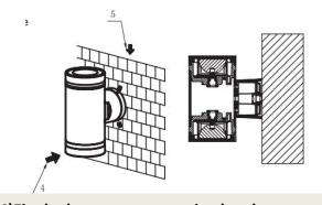
4) Fix the lamp onto mounting bracket
