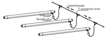
3. Install Sign LED Tube in place(bracket) and connect the Input AC wire as shown below.
